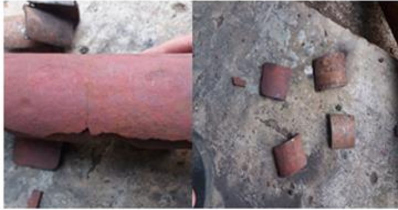
Figure 4. Pipe pieces that have undergone combustion activity
