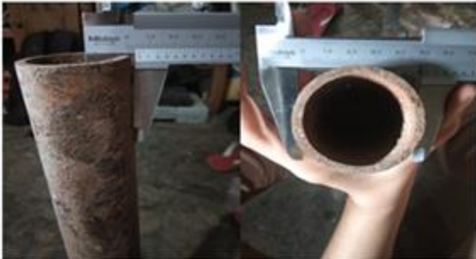
Figure 2. Size of pipe material before and after corrosion
