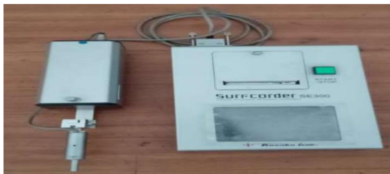
Figure 2. Measuring tool roughness (surface tester)
