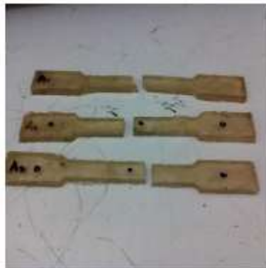
Figure 7. Pure Resin Specimen After Testing
