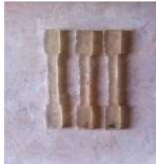
Figure 6. Pure Resin Specimen Before Testing
