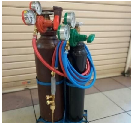
Figure 2. Oxy acetylene welding machine
