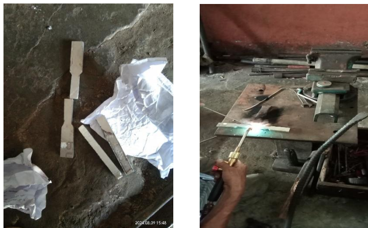
Figure 5. Welding specimen a). specimen before welding b). welding process at the joint specimen Source: Personal Documentation (2025)
