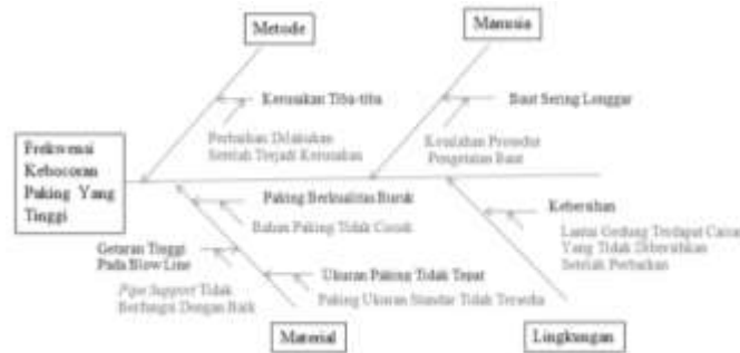
Figure 6. Fishbone Diagram Causes Gasket Leakage Frequency Tall
