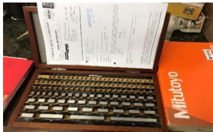
Figure 2. Mitutoyo Gauge Block (0-200 mm) with certificate
