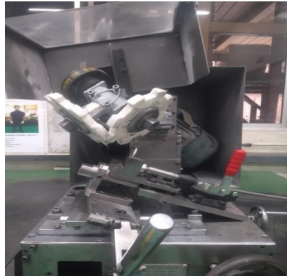
Figure 4. Profile Point Hook Grinding Machine at PT. XYZ
