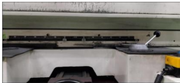
Figure 8. Setting the stopper using an assembly block
