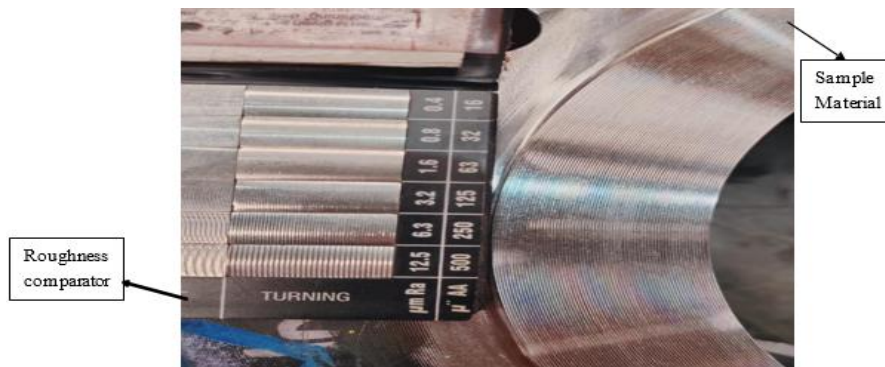
Figure 4. Raise face flange surface roughness measurement
