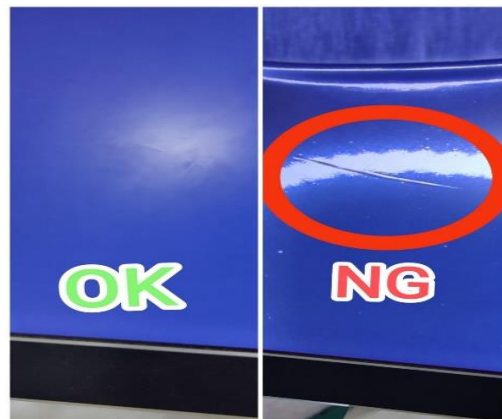
Figure 4. Flow mark defects
