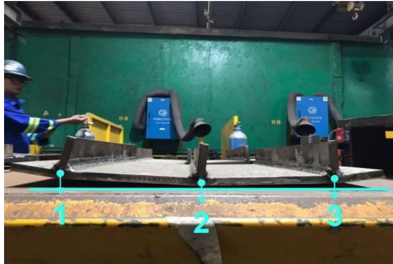
Figure 6. Results of the string welding sequence process
