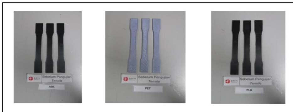
Figure 3. Tensile Test Specimens: (a) ABS, (b) PET, (c) PLA
