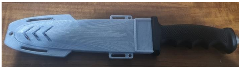
Figure 9. Bayonet sheath printed using recycled PET filament
