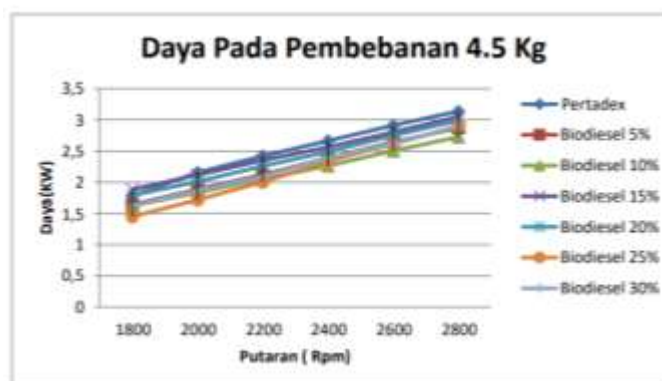
Figure 4. Power vs Speed Graph for 4.5 kg . load
