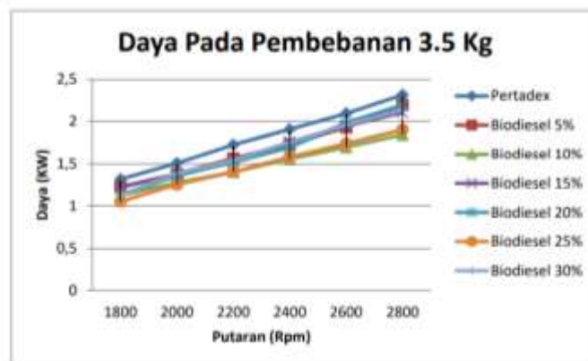
Figure 3. Power vs engine speed graph for 3.5 kg beban load
