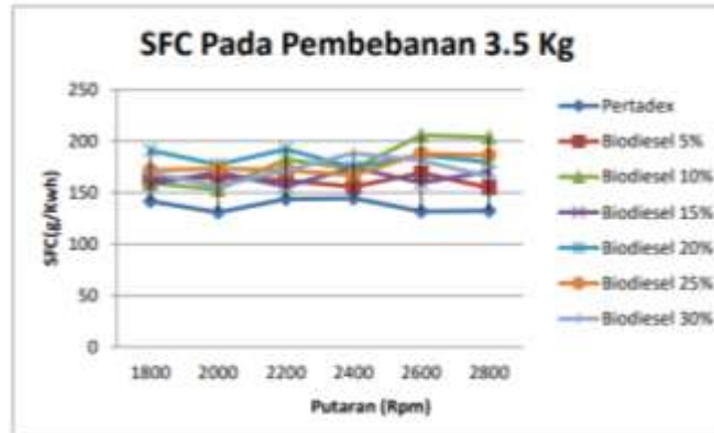
Figure 7. SFC vs Engine speed at 3.5 kg load
