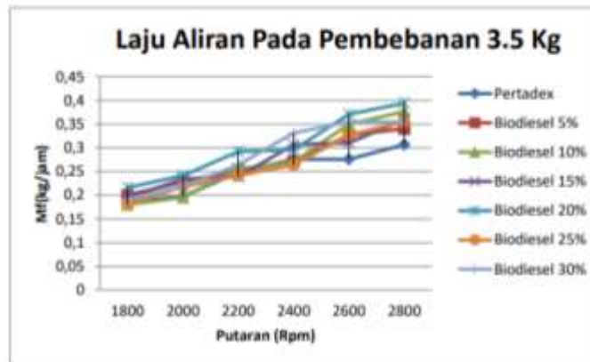
Figure 5. Graph of mf vs. engine speed for a load of 3.5 kg
