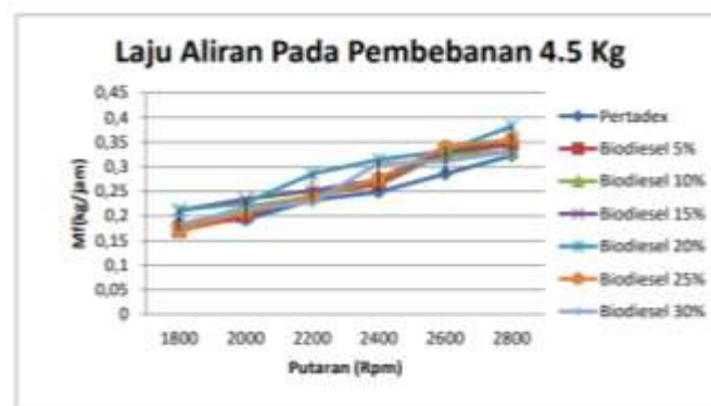
Figure 6. Graph of mf vs. engine speed for a load of 4.5 kg
