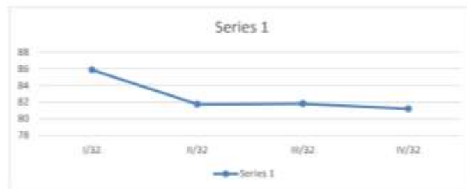
Figure 2. Graph of the average hardness value (HRB) with an E 308L electrode with a diameter of 3.2 mm
