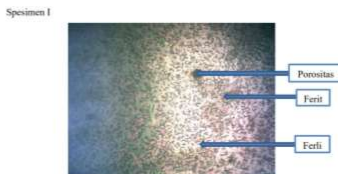
Figure 4. Microphotographs with E 308L electrodes with a diameter of 2.6 mm and a current of 85 A
